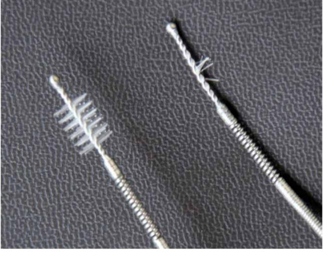
Figure 1: New brush (left) and old brush (right)
