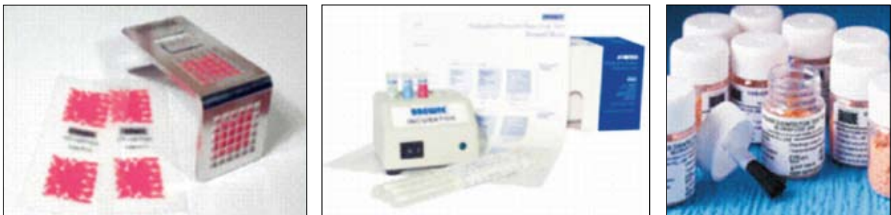
Figure 1: A cleaning indicator (left), cleaning endpoint test kit (based on a swab test using ninhydrin; middle) and artificial test soil (right) for use in the monitoring of cleaning processes.
