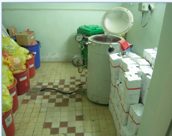
Figure 2. Typical waste sampling room in a hospital in Ulaanbaatar with steriliser for sharps, not working, but still kept for inspections
