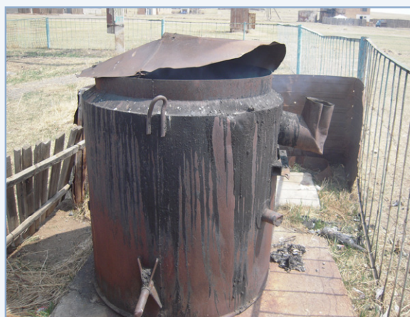
Figure 3. Typical self constructed waste incinerator in a soum hospital
