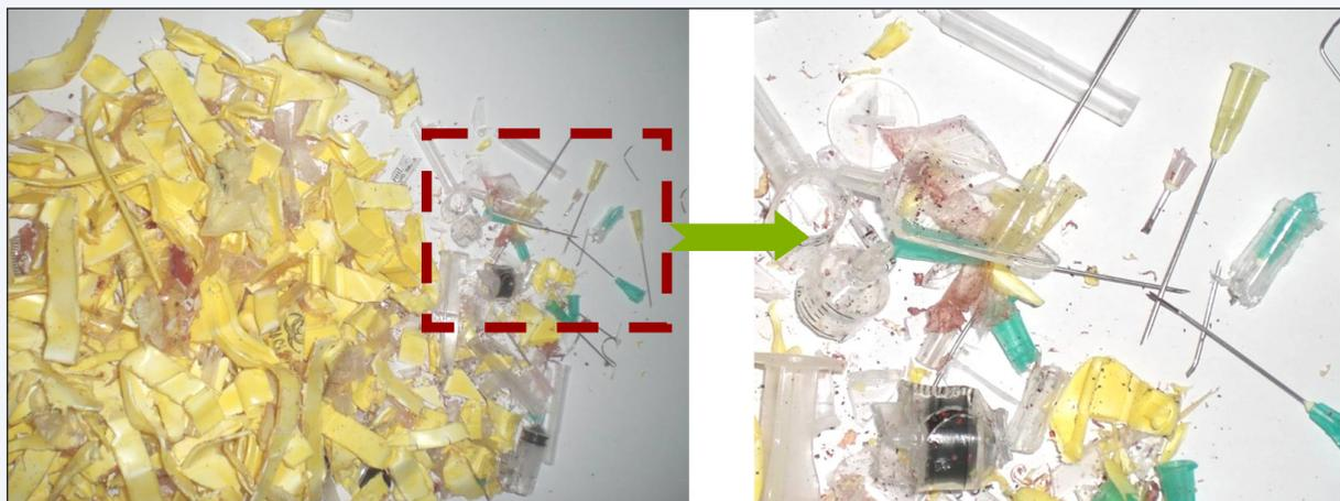
**Figure 1: Sharp boxes after shredding. Needles are, if at all, only partly cut or bended.**
