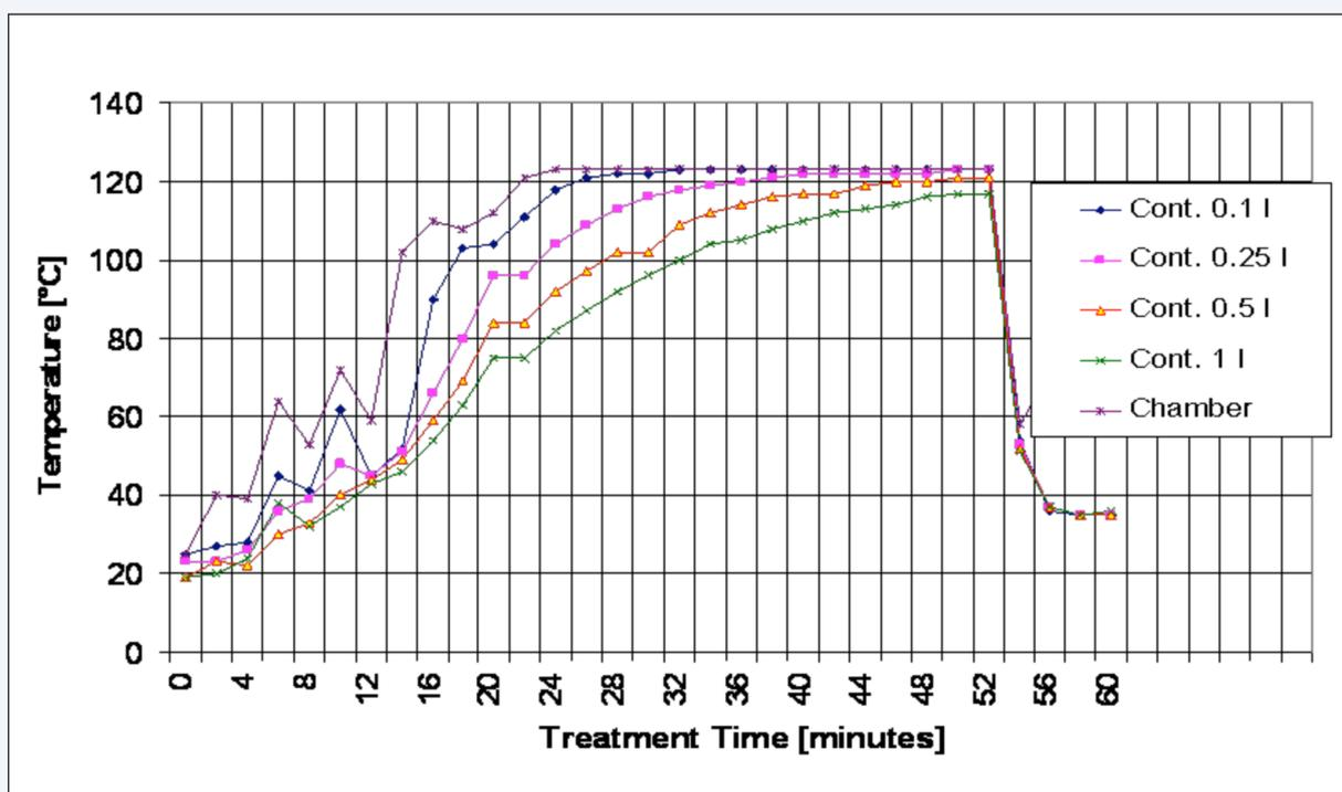
**Figure 6: Actual treatment temperatures in liquids of different volumes during a typical, bio-hazardous waste treatment cycle of an advanced waste treatment autoclave.**
