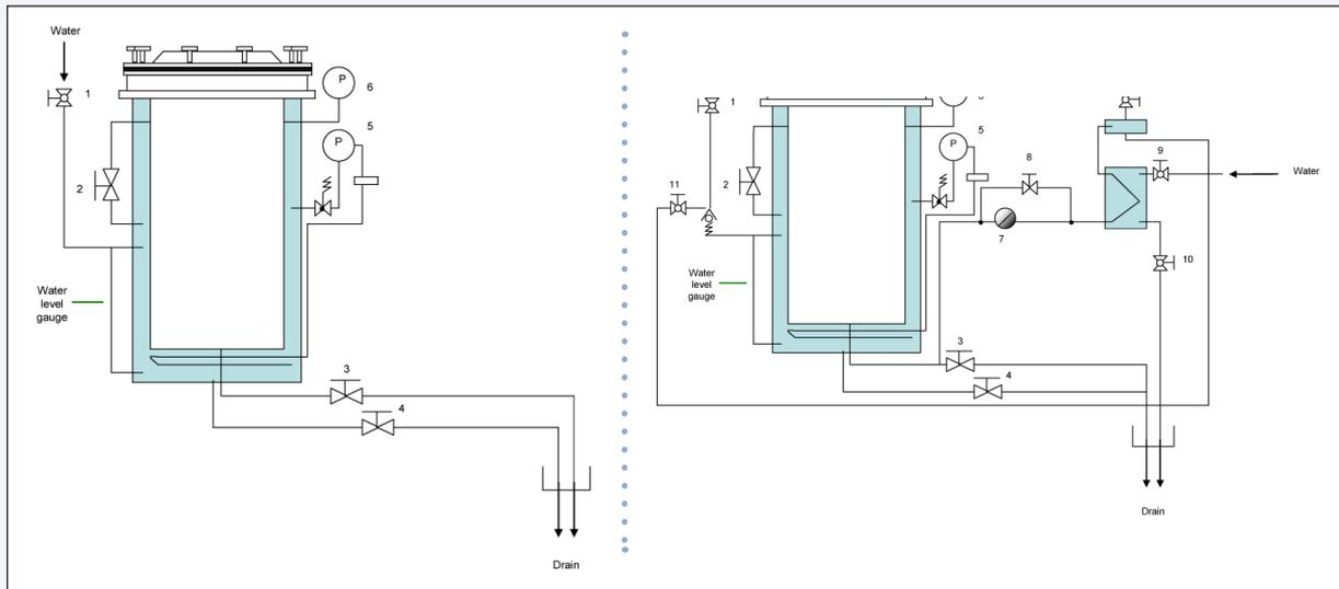
**Figure 4: P&I Diagram of an old autoclave (1) and with added condenser and HEPA filter (2)**
