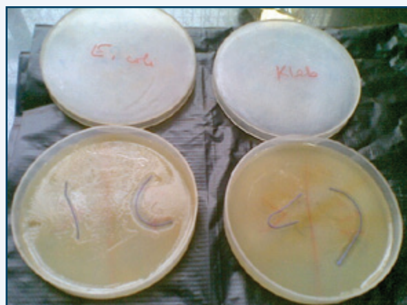
Figure 3. Good zone of inhibition around coated suture, no zone of inhibition around uncoated suture against Acinetobacter , E. coli and Klebsiella spp.
